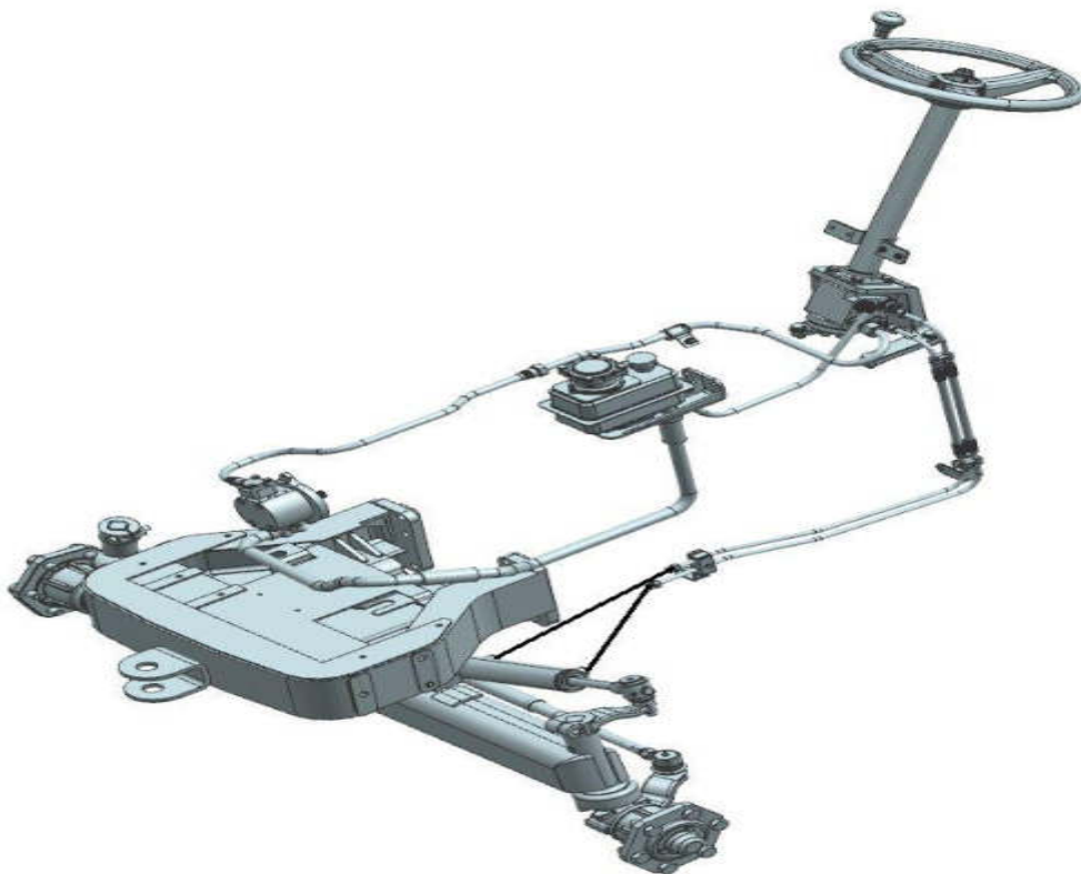
Fig 2: OPTIONAL FITMENT: HYDROSTATIC POWER STEERING
